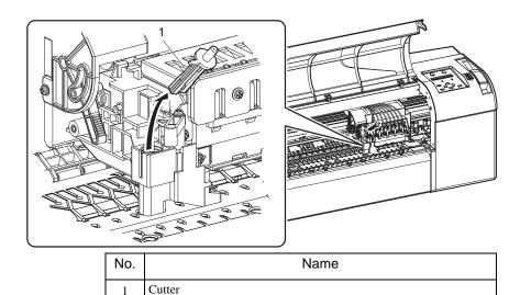
9. Attach the new cutter as shown in the illustration.
