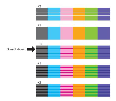
• After micro adjustment printing is completed, "PF Adjust: Micro Print" is displayed on Operation panel.
