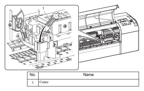
10. Gently push the knob of the razor blade and reposition the cutter holder lever simultaneously.
